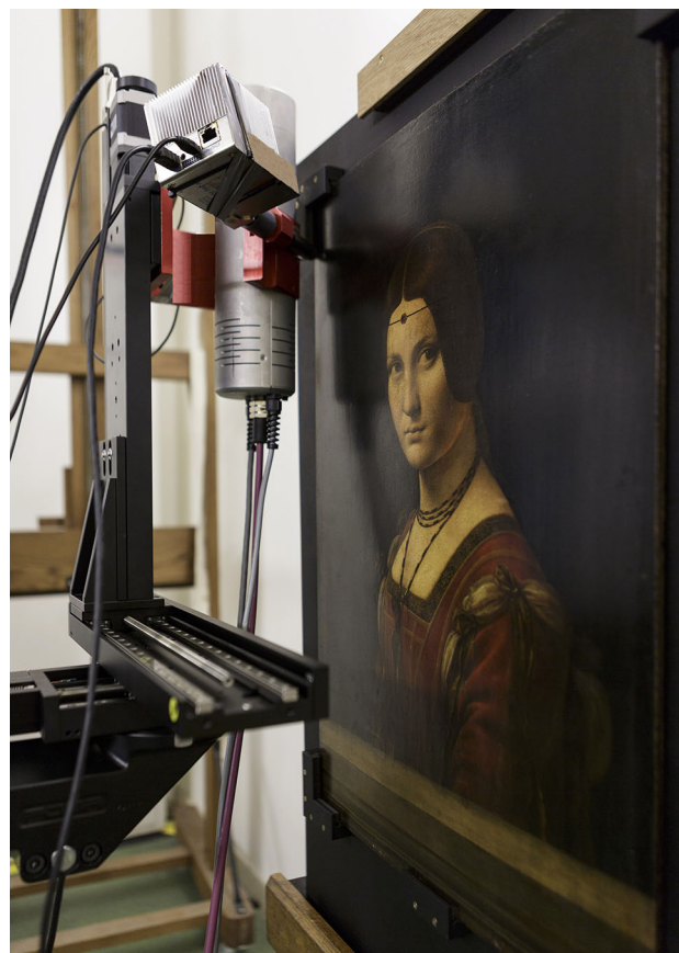
Fig. 1 MA-XRF instrument in front of the Belle Ferronnière by Leonardo da Vinci (1452–1519), Musée du Louvre, INV. 778
