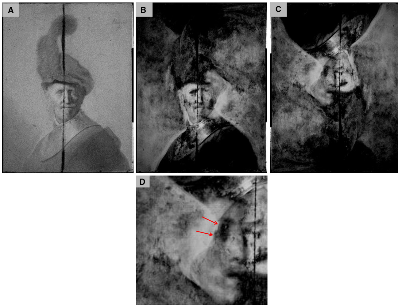
Fig. 2 a MA-XRF Pb-M \alpha element map; b Pb-L \alpha element map; c Pb-L \alpha element map, rotated 180° to better show face and cloak of underlying man; d enlargement of area in c of face of underlying figure, with arrows pointing to the two eyes
