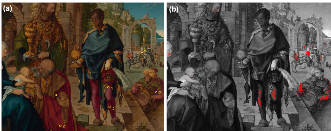
Fig. 8 RGB colour image of the Adoration of the Magi (a) and map of the painting considering a parabolic fit in the 519–544 and 558–580 nm ranges (b), reconstructed from the cube files
