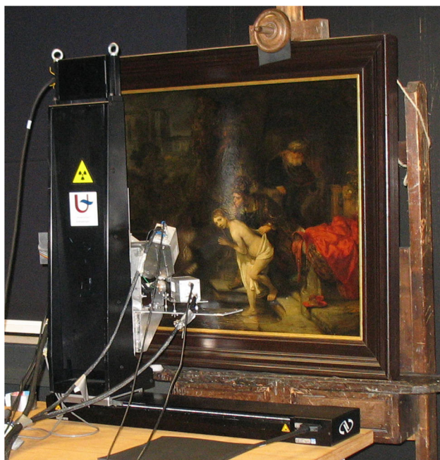
Fig. 2 MA-XRF scanner during investigation of Susanna and the Elders in the conservation studio of the Gemäldegalerie, Berlin
