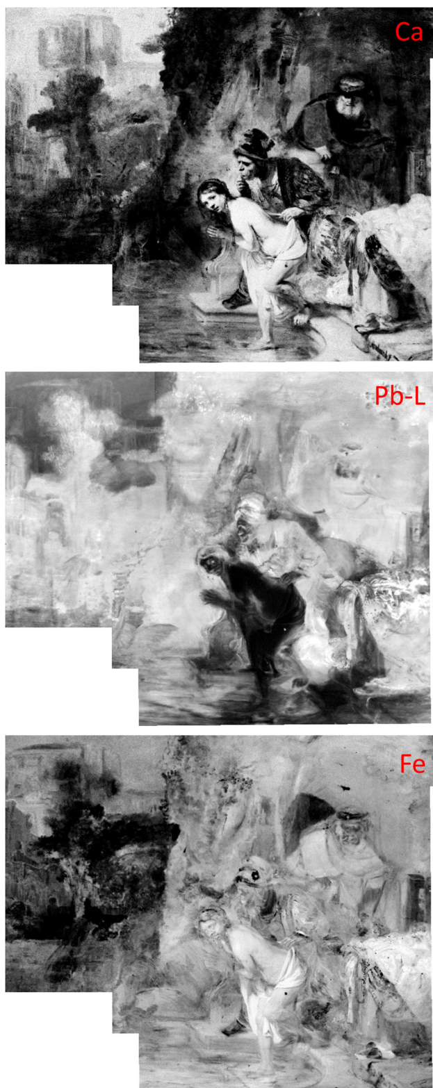
Fig. 5 Elemental distribution images of Ca, Pb and Fe acquired by MA-XRF
