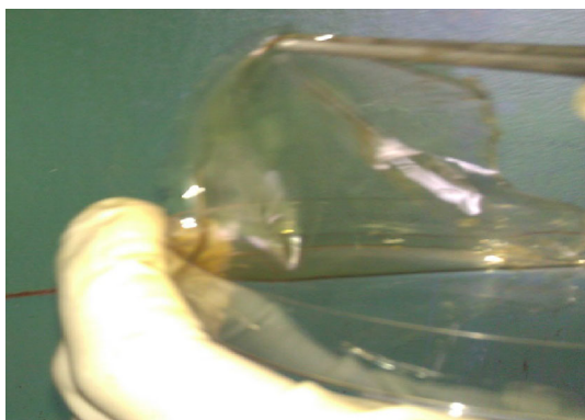
Fig. 8 Standing film formed from the polymer electrolyte
