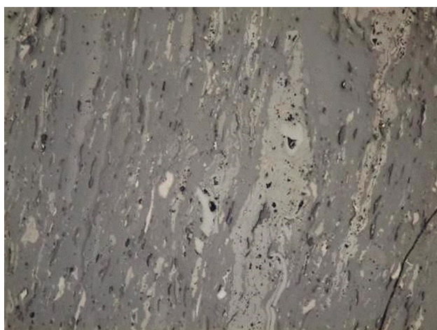
Fig. 1 A thin section of a coal sample in reflected light. Macerals of the inertinite, vitrinite and liptinite groups have black, pale grey and grey colours, respectively. The micro and nanoscale pores are also present in the sample
