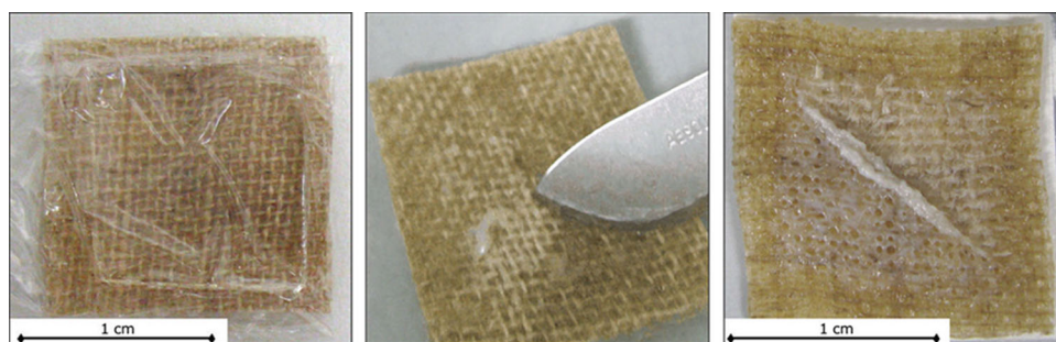
Fig. 4 Application of H50 hydrogel on the canvas glued with Plextol ® adhesive, which, after swelling, could be removed by gentle mechanical action ( left and center ); removal of Mowilith ® adhesive after application of H65 hydrogel ( right )
