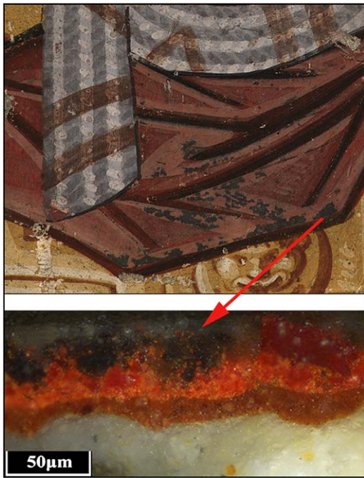
Fig. 1 Minium alteration detected on red garment (Protaton wall paintings) [13]
