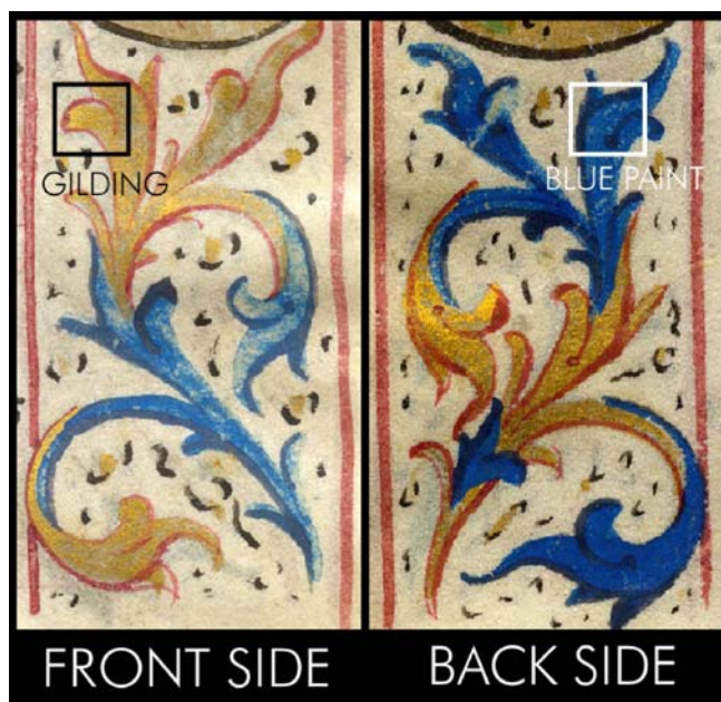
FIGURE 11 Left : a detail of the gilded area where a \mu -XRF spectrum was collected (data in Fig. 12). Right : the same area on the back side of the parchment with blue paint. Signals from the gilding and the blue paint appear in the \mu -XRF spectrum
