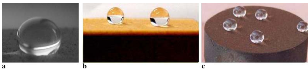
FIGURE 1 Optical images of a few water droplets on the surface of the PEEK/PTFE composite coating at different curing temperatures: (a) at 25 °C; (b) at 200 °C; (c) at 300 °C
