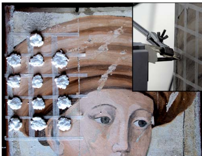
FIGURE 1 Painting on mortar (mock-fresco), coated with polymer, and with microemulsion compresses applied. Detail of fiber-optic reflectance probe-head measuring the sample surface (top right)
