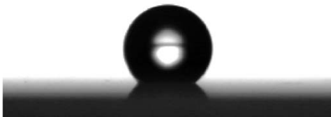
FIGURE 2 The water contact angle on the surface of thin film as prepared. Contact angle of water 146.8°
