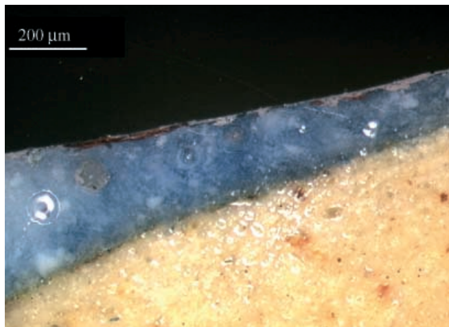
FIGURE 8 Optical microscopy image acquired from a polished section obtained from a lustrated ceramic shard: the ceramic body ( bottom ) and the glaze ( top ) decorated with the blue pigment smalt are visible
