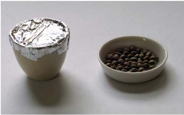
**Fig. 1** The crucibles used, one covered by aluminum foil, the second left open
