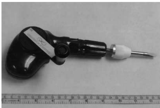
Fig. 2 Magnetic resonance-compatible manually driven 4.5-G titanium drill
