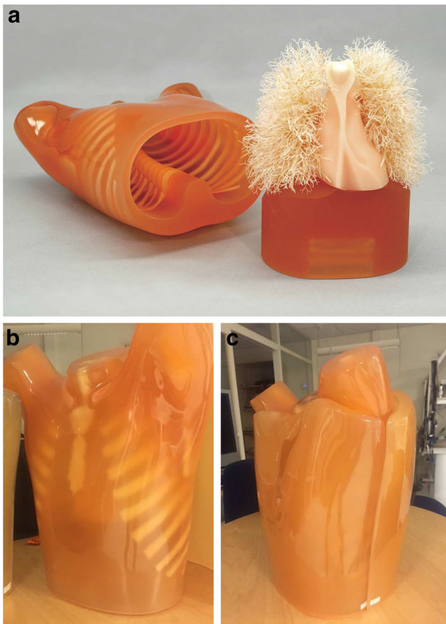
Fig. 1 a The abdominal block removed from the Lungman phantom. b The torso simulating a male of approximately BMI 23 (chest girth 94 cm). c The torso with added chest plates simulating BMI 29 (chest girth 112 cm) [15]
