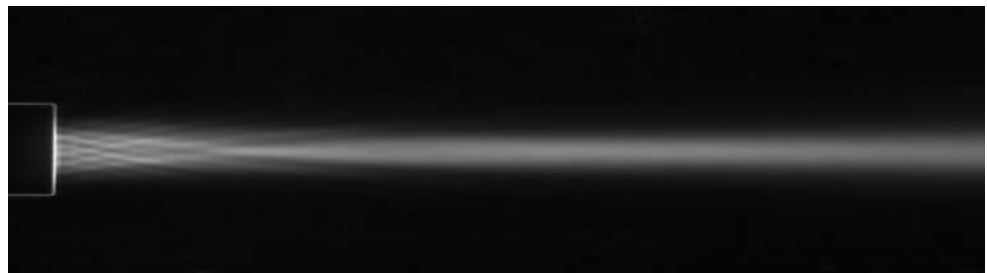
Fig. 2 Picture of the ultrasound wave emitted by a piezoelectric probes at 1.25 MHz
