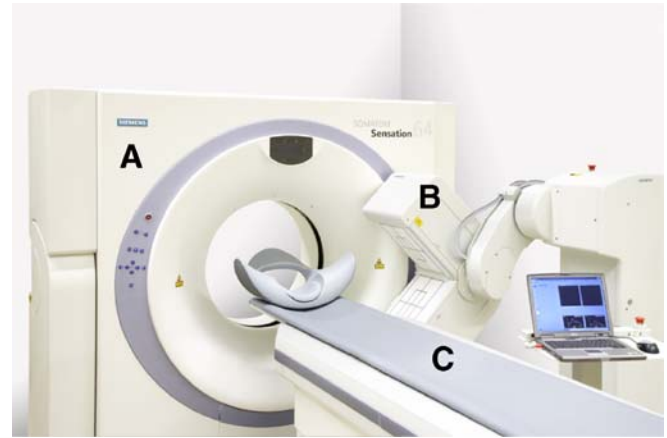
Fig. 2 Integrated instrumental setup of a 64-slice MDCT system (A) with a retractable SPECT camera (B) which can be attached to the CT patient table (C) from its storage position when active via a rail-track (not visible) in the room floor
