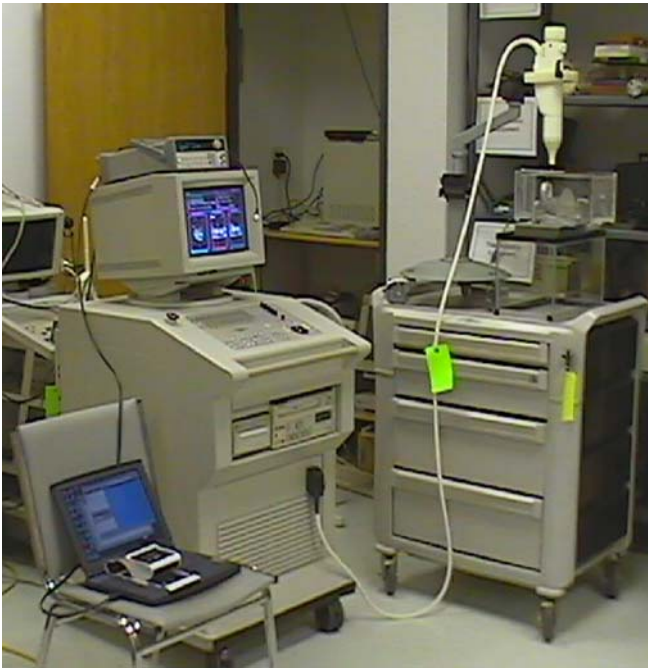
Fig. 1 Modified Sonablate™ 200 with ultrasound probe. Experimental setup of the single components ultrasound transducer, high frequency amplifier, diagnostic and therapeutic ultrasound probe and experimental water bath
