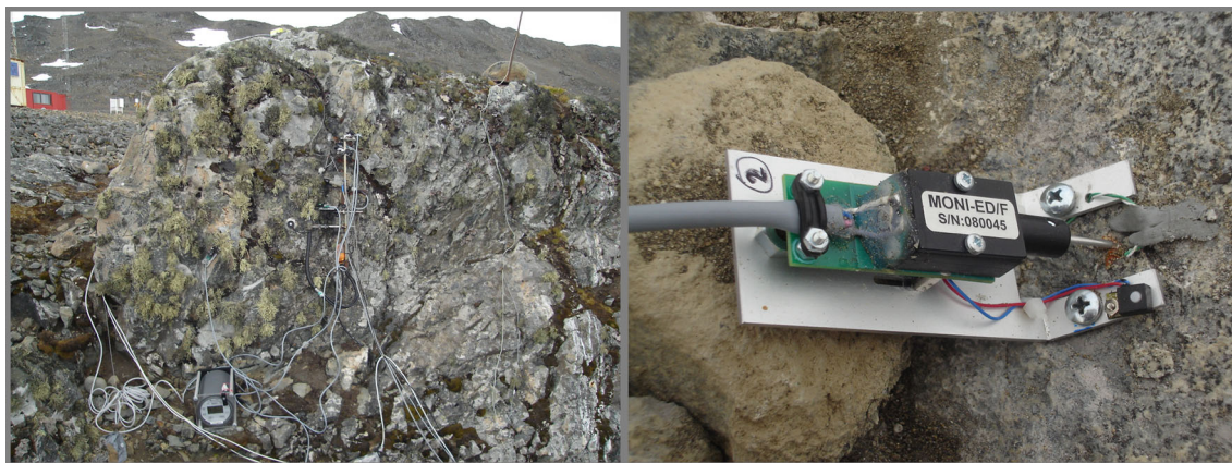
Fig. 2 MoniDA working in Livingston Island, maritime Antarctica ( left ) and an individual probe with fluorescence, temperature and light sensors monitoring Caloplaca sp. in Garwood Valley, McMurdo Dry Valleys, Continental Antarctica ( right )
