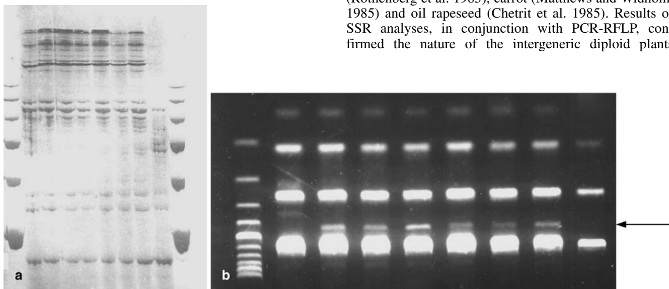
Fig. 4 Analysis of mitochondrial genome of the intergeneric diploid plants by PCR-RFLP with primer-enzyme combinations nad4 ex 1–2/ TaqI ( a ) and nad4 ex 1–2/ HindIII ( b ). a Lanes (from left to right): DNA size marker, M. papuana Swingle, regenerated plants
