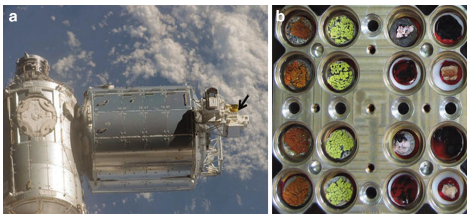
Fig. 5 Experiment hardware and biological samples of the LIFE experiment. a EXPOSE-E facility (black arrow) outside the Columbus module of the ISS during orbital flight, accommodating the LIFE samples. b Samples of the LIFE experiment (lichens and Antarctic RIF) accommodated in one of the compartments of the EXPOSE-E facility (Scalzi et al. 2012)
