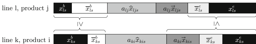
Fig. 4 Production of successor product j on line l must neither start nor end before predecessor product i on line k in every microperiod s .
