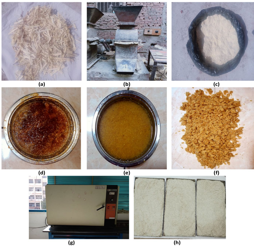
Fig. 1 The alkali treatment process of extracted sugarcane bagasse fibers
