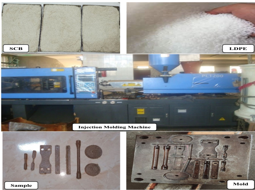
Fig. 2 The fabrication steps for injected composites
