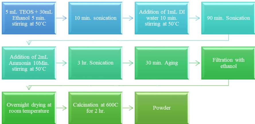
Fig. 7 Flow diagram of preparation of silica nanoparticles using calcination process [34]
