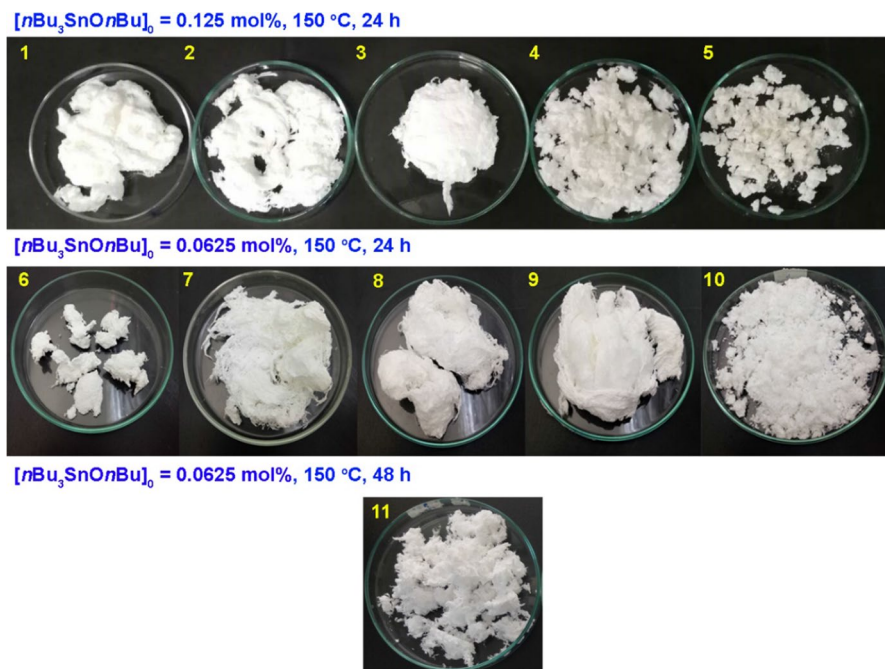
Fig. 6 Physical appearances of the synthesized PCLs (entries 1–11) from the ROP of \epsilon -CL with the n\text{Bu}_3\text{SnOnBu}/\text{Al}(\text{OsBu})_3 mixed initiators at 150 °C for 24 and 48 h
