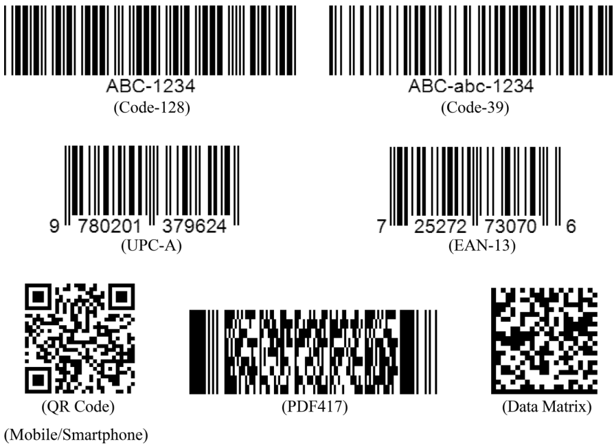
Fig. 4 Some barcode models in general (All codes are created by the author, https://barcode.tec-it.com/en )
