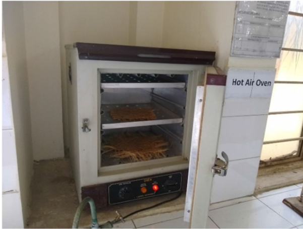
Fig. 1 Heat treatment of fibers in a hot air oven
