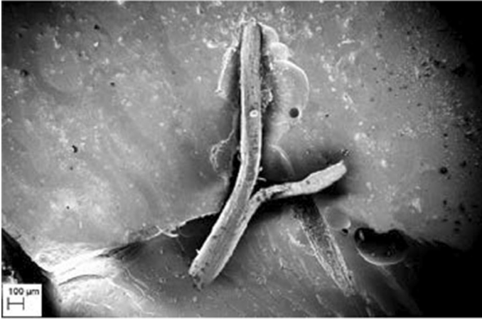
Fig. 10 Untreated coir fiber specimen showing loose bonding and slippage
