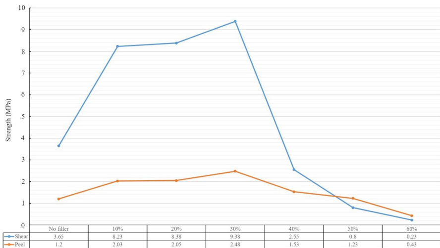
Fig. 18 Variation in shear and peel strength with filler volume fraction [141]
