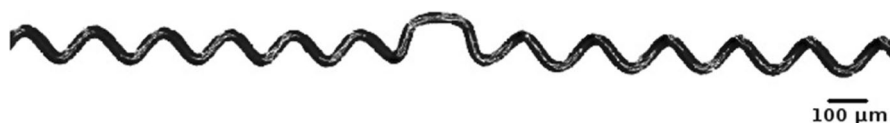
Fig. 4 Perversion observed in the process of curling and wrinkling of an electrospun fiber (authors' image)
