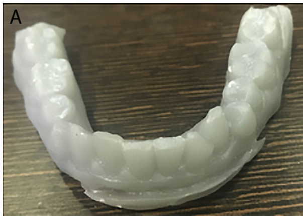
Fig. 7 Polyjet printed dental long-term (LT) resin-based clear aligners (with kind permission from Elsevier publisher [69])
