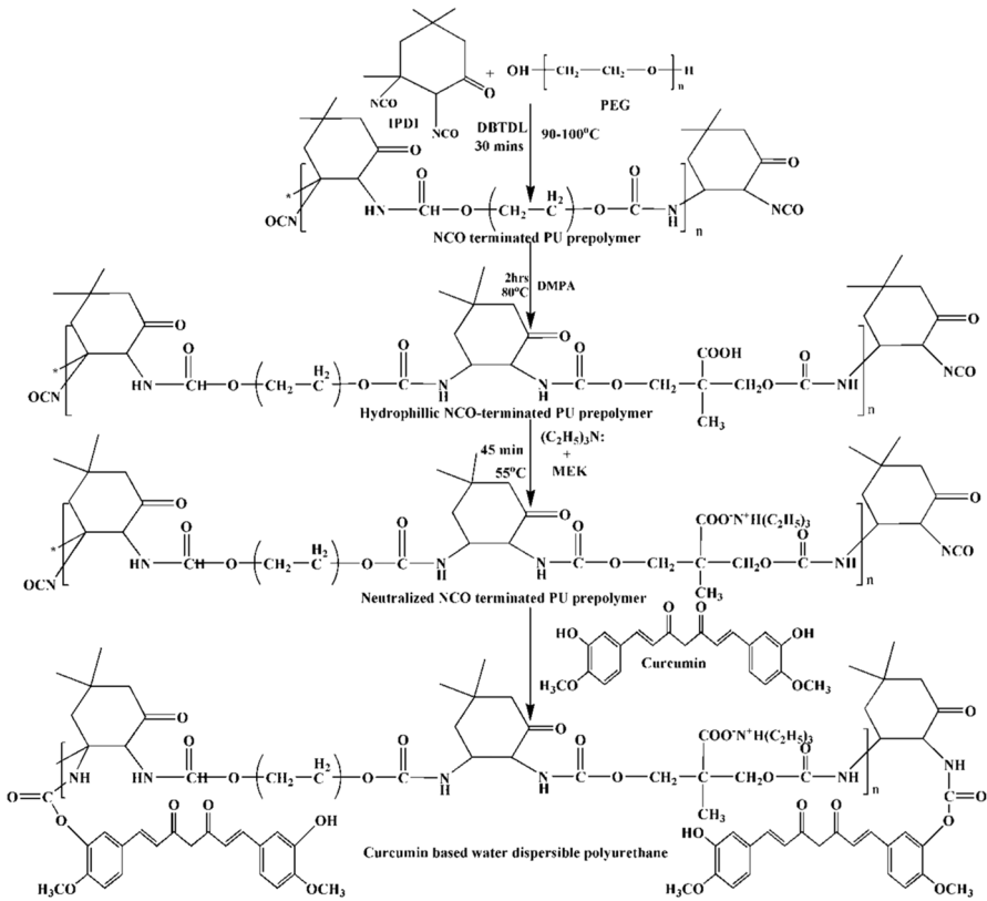
Fig. 1 A schematic illustration of the synthesis of curcumin-based water-dispersible polyurethane
