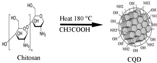
Fig. 1 Schematic for the synthesis of carbon quantum dots from chitosan
