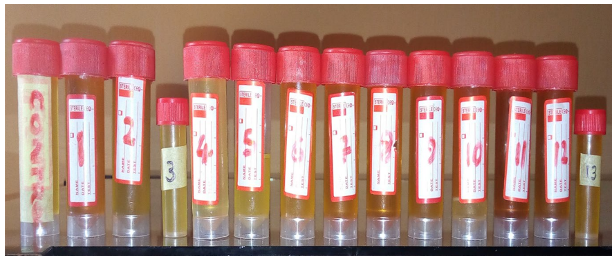
Fig. 3 Mixed waste plastic pyrolysis liquid samples. Source: Eze et al. [23]
