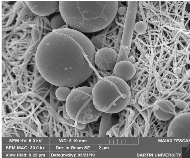
Fig. 3 SEM image of PET nanofibers/CuO nanoparticles
