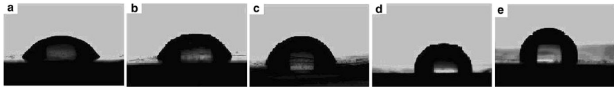
Fig. 6 The contact angle of a PU0, b PU10C, c PU2, d PU6 and e PU10
