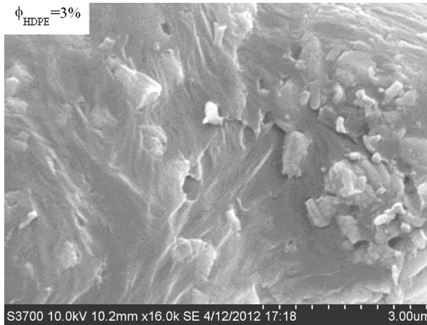
Fig. 10 SEM photograph of impact fracture surface of POM/EVA/HDPE/nano-CaCO 3 composites ( \phi_{HDPE} = 3\% )
