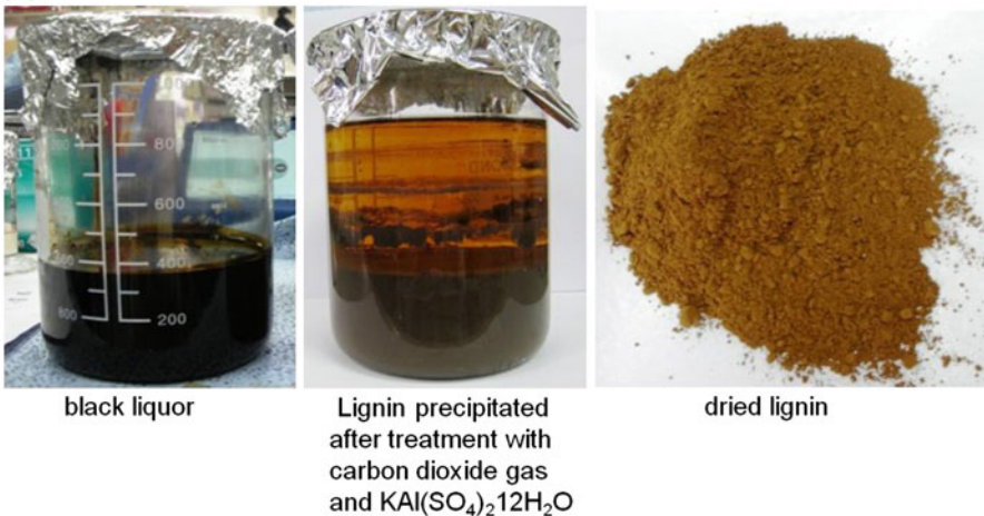
Fig. 1 Extraction procedure of lignin from black liquor (a) and digital camera images of black liquor precipitates and dried lignin-SKKU (b)
