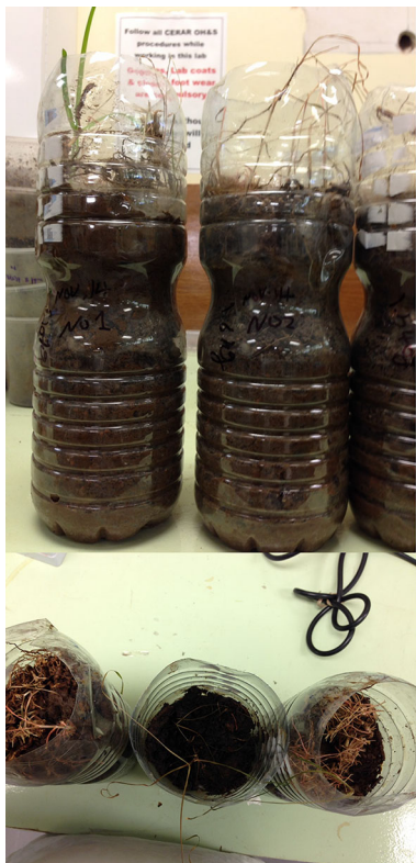
Fig. 1 The soil columns after contamination with crude oil
