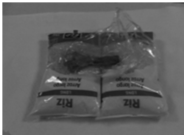
Fig. 1 Specimen positioning using rice bags to simulate soft tissues and get a reproducible position through the experimental protocol
