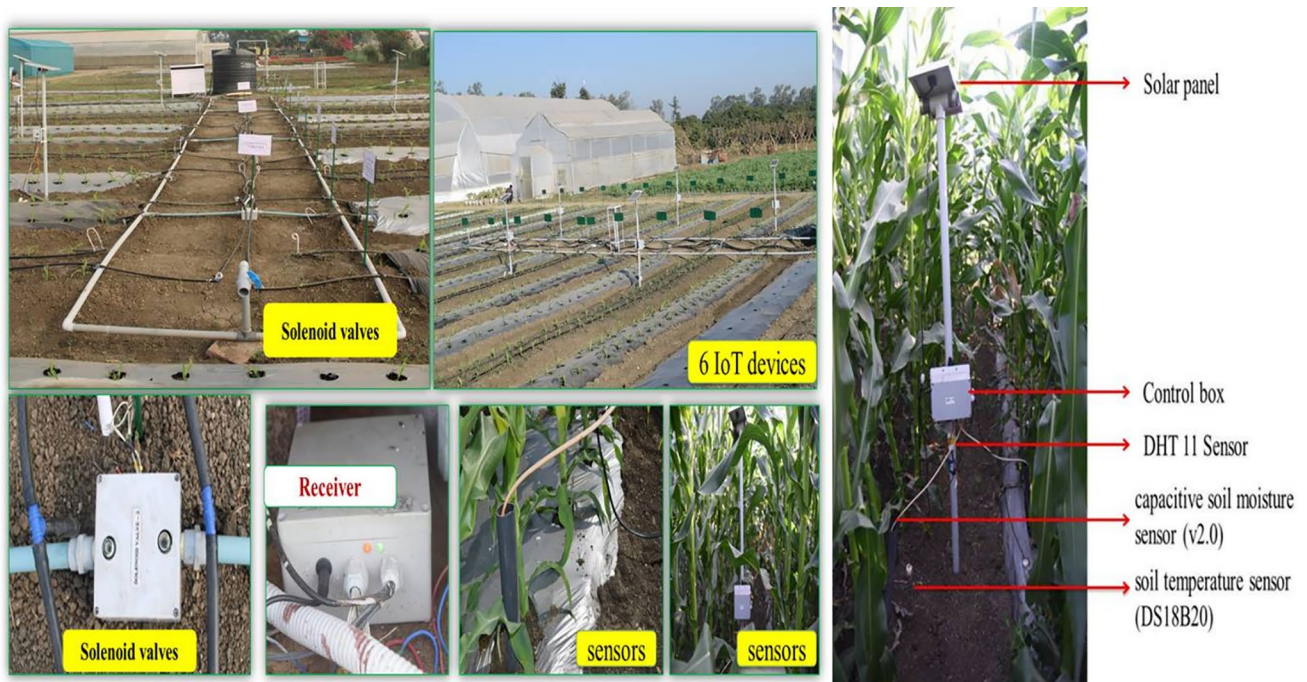
Fig. 8 IoT-based wireless data monitoring systems in a full-scale field experiment
