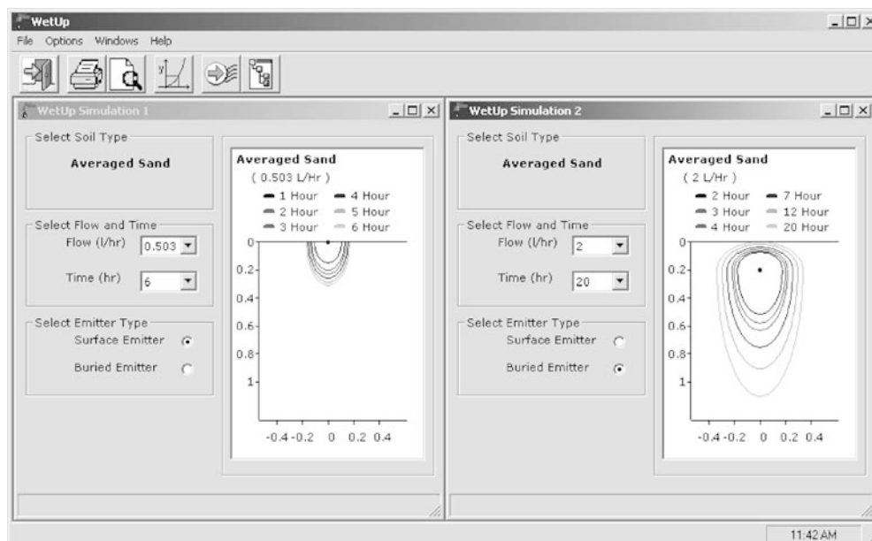
Fig. 1 WetUp window showing wetting perimeters at different times for different flow rates from a surface emitter (panel 1) and buried emitter (panel 2)
