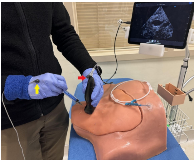
Fig. 1 Laboratory setup of the experiment: The first hand motion sensor placed on the dorsum of participant's right hand (yellow arrow), and the second on the base of the US probe (red arrow). Note, actual recorded video was limited to the participant's hands
