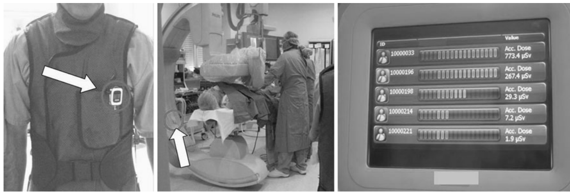
Fig. 1 Detector over the specialist apron ( left ). Detector located at the C arm to have an estimation of radiation dose without protection ( center ). Base station displaying different levels of radiation with a color code
