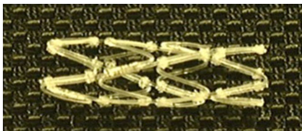
Fig. 1 Biodegradable stent. Monopolymer PLLA filaments are arranged in cylindrical zigzag form, 6 mm in diameter and 15 mm in length, with a marker to check position under fluoroscopy
