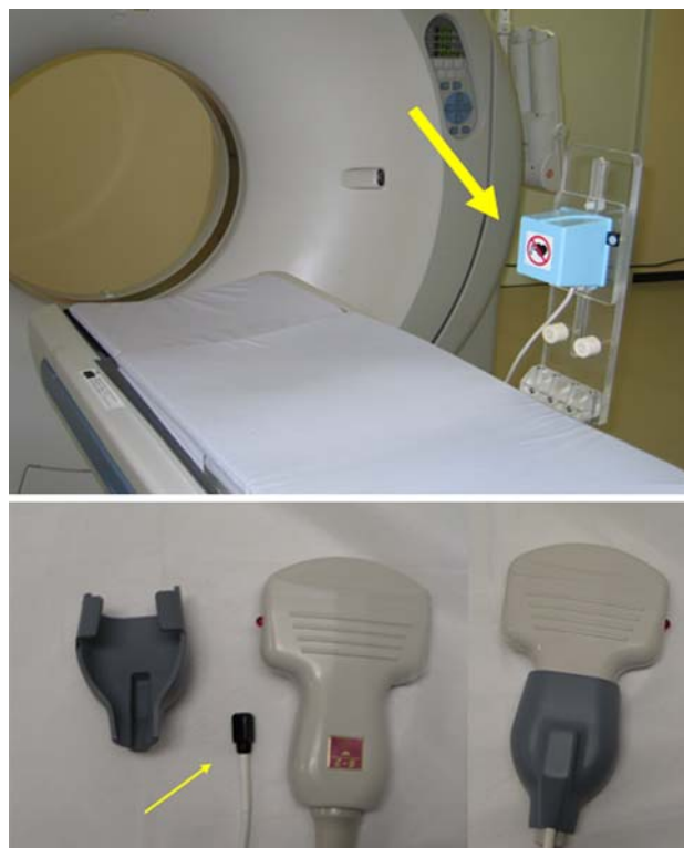
Fig. 1 Real-time virtual sonography at the time of RFA treatment. The transmitter was fixed to the CT stage ( thick arrow ), and a magnetic sensor was applied to the sonographic probe ( narrow arrow )
