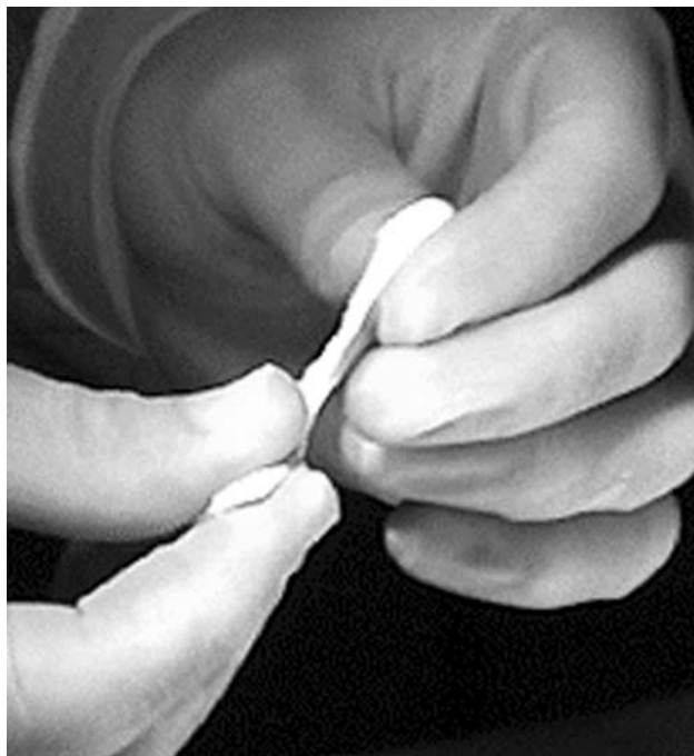
Fig. 2 After mixing, the high-viscosity bone cement showed the consistency of Plasticine (putty-like)
