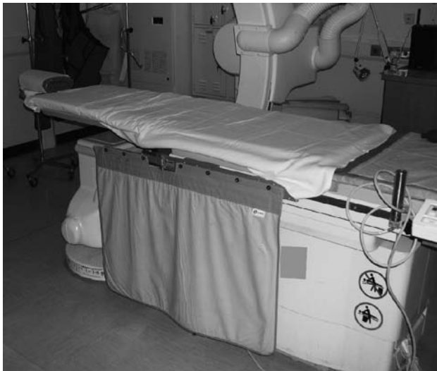
Fig. 1 Protective lead curtain along the side of an interventional fluoroscopy table
