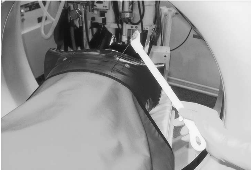
Fig. 1. Measurement of radiation dose to the radiologist's hand by using the Alderson phantom. Radiation protection tools with placement of lead drape 2 cm caudally from the central plane and use of radiation protection gloves and long needle holder.
