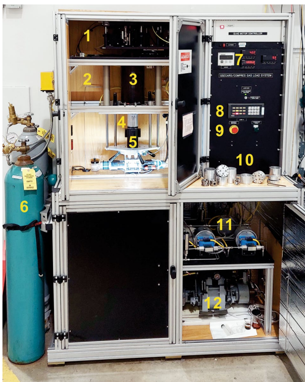
Fig. 15 The GSECARS and COMPRES jointly funded gas-loading system for diamond anvil cells located adjacent to experimental station 13-ID-D. The system can load many kinds of diamond anvil cells with a closure mechanism using motor driven screws which close a clamping device, not the cell itself. This design makes it easy to pressurize new cell designs using a different clamp or different spacer. The system has optical access for sample viewing and online ruby fluorescence pressure measurement. 1=Microscopy and ruby fluorescence system; 2=Pneumatic cylinder; 3=Pressure vessel; 4=Diamond anvil cell clamp; 5=Vessel bottom plug; 6=Gas supply tank (He, N 2 , Ne, Ar, Xe, or CO 2 ); 7=Pressure gages; 8=Control panel; 9=Emergency stop button; 10=Gear boxes for various DACs; 11=High pressure valves; 12=Compressor
